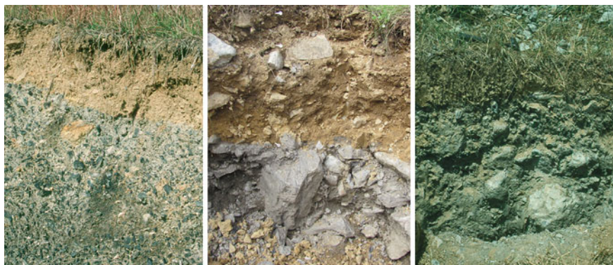
Fig. 6 Profiles of mine soils constructed with controlled placement of “topsoil” salvaged as mixtures of the original A horizon with subsoil materials having been placed at <0.5-m depths over rock spoils (left and center) and placed at greater depth (right) (Photos by Jeff Skousen)
