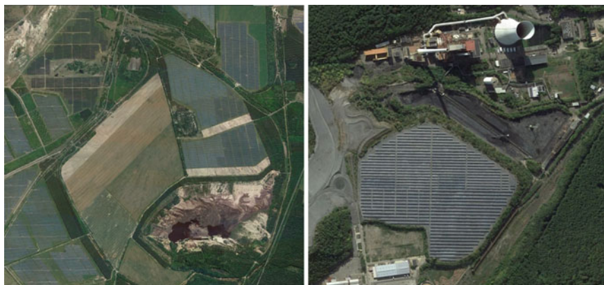
Fig. 6 Photovoltaic energy facilities, “solar farms”, constructed on mined land in Europe (Left) An 8.4 MW solar array constructed on approximately 20 ha of coal-mine spoils near Goettelborn in western Germany; (right) One segment of a 168 MW photovoltaic facility constructed on lignite mine spoils near Senftenberg in eastern Germany. (Photos from Google Earth)
